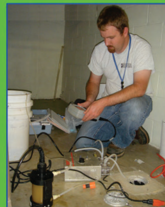
Examples of flow cell monitoring for groundwater contamination reporting purposes both indoors and outdoors.
