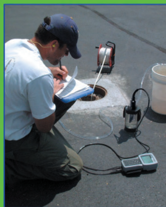
Examples of flow cell monitoring for groundwater contamination reporting purposes both indoors and outdoors.
