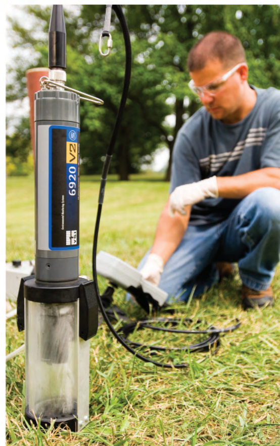
Wiped fouling protection for DO, pH, ORP, and turbidity sensors ensures accurate data collection.
